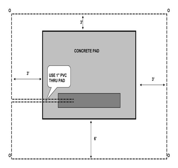
GROUNDING GRID 1/0 BARE COPPER BURIED 6" BELOW FINAL GRADE, RUN WIRE THRU 1" CONDUIT WITH 5' TAILS INTO TRANSFORMER PAD.
